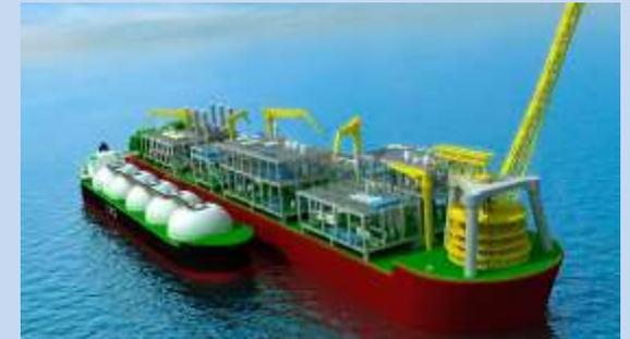
Prelude has decks 488 metres long and 74 metres wide. The ship weighs more than 600,000 tonnes fully ballasted - roughly six times as much as the largest aircraft carrier. Some 260,000 tonnes of that weight will consist of steel - around five times more than was used to build the Sydney Harbour Bridge.
